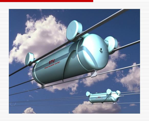
The most important innovation which insures low cost, reliability and scalability of the system is introduction of coupler cable drive to propel dump-cars. Coupler cable performs few functions which enables to reduce cost and increase reliability of the system, specifically:
