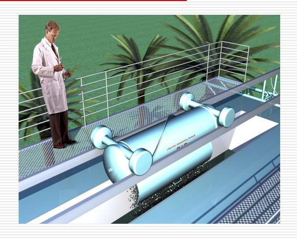
Rolling stock is highly aerodynamic dump-cars. These dump cars are inexpensive non self propelled vehicles, much like railway cars.
