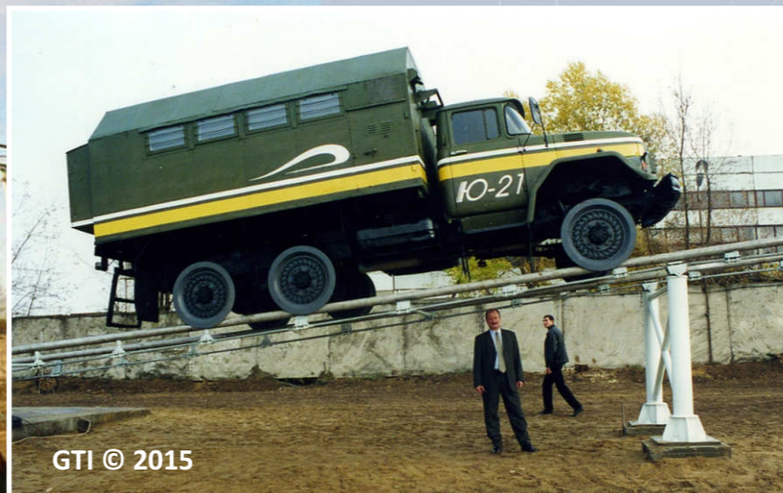
A.Yunitskiy demonstrates viability of track structure standing under a 15 ton truck ZIL-131
